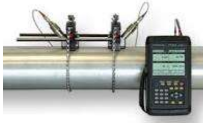
Water flow meter
