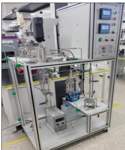
Figure 5-3. Internal Circulation Mineral Carbonation Reactor (lab scale)
