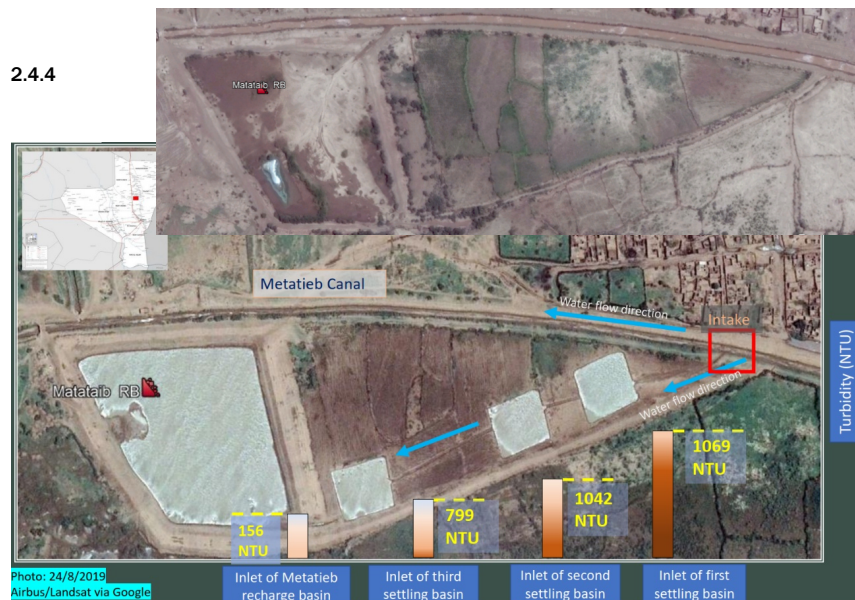
Figure 12. Aerial views of the Matateib artificial recharge system in North Delta, Kassala State. The upper image shows the Matateib recharge basin and nearby agricultural plots along the Gash irrigation canal. The lower annotated image illustrates the sediment pre-treatment system introduced under the project: an elongated diversion canal with three sequential stilling basins (each 50 × 50 m, 1 m deep) designed to slow flow and trap sediment before water reaches the recharge basin. Turbidity values measured at each stage (1069 → 1042 → 799 → 156 NTU) confirm an 80% reduction in suspended load, demonstrating the system's effectiveness in minimizing basin clogging and extending operational life.
