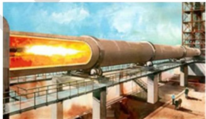
**Fig1. Cement kiln use waste tire as alternative fuel**
