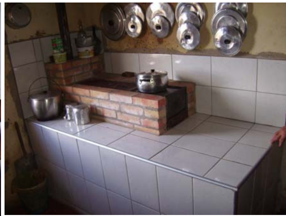
Improved cook stove of IDER; original design (above left) and improvements introduced by the users
