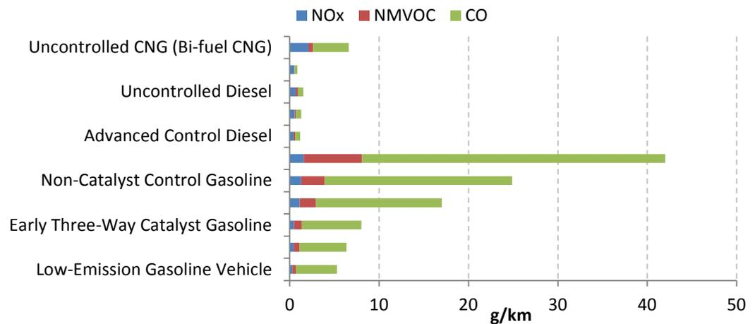
Figure 7. Vehicle operation emissions of CNG, diesel and gasoline technologies.
