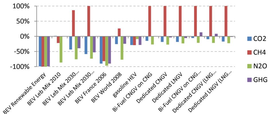
Figure 5. WTW GHG emissions change of NGV, gasoline HEV and BEV comparing to 2010 conventional vehicle.
