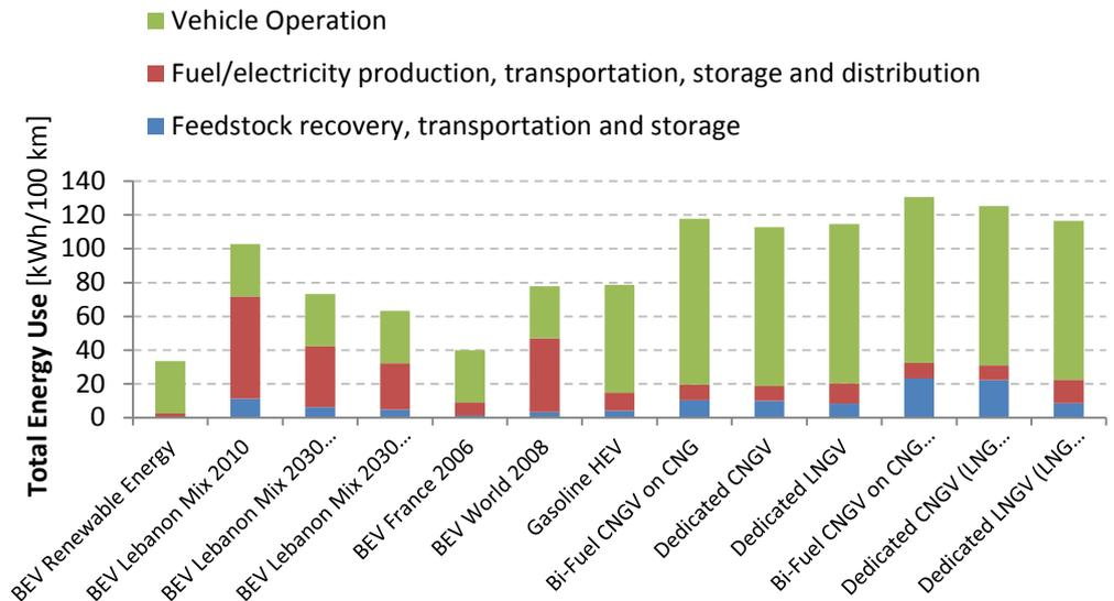
Figure 4. WTW total energy use of NGV, gasoline HEV and BEV using different electricity generation mix.
