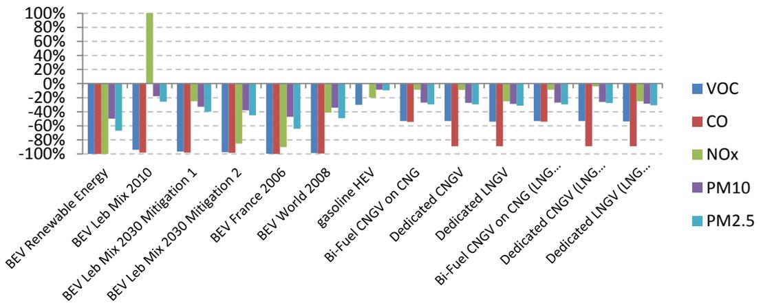
Figure 6. WTW pollutants change of NGV, gasoline HEV and BEV comparing to 2005 conventional vehicle under urban driving conditions.
