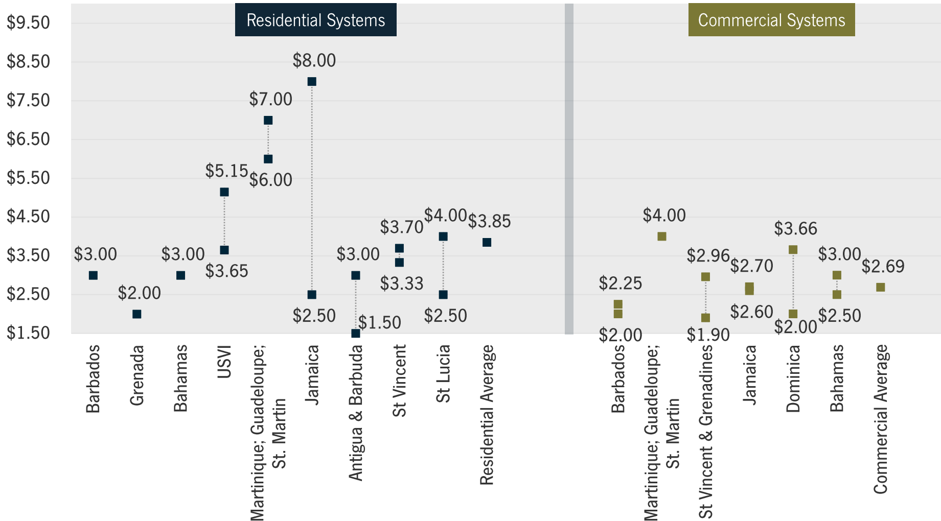
Range of Distributed Generation PV System Pricing (USD/W)
