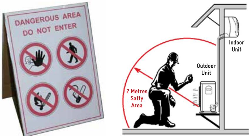
Figure 5: Designated work area where potential Sources of Ignition (SOI) must not be present during service works
