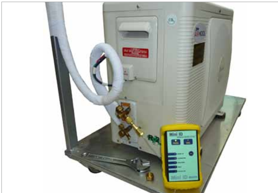
Figure 6: Example testing the "old" existing HCFC R22 refrigerant quality
