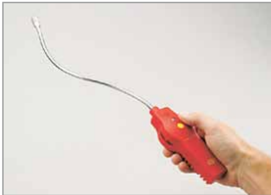
Figure 33: Leak check with electronic leak detector
