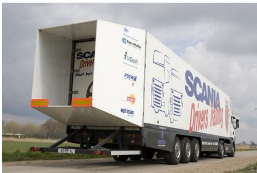
Figure 19: A 'boat tail' prototype as developed by the Platform for Aerodynamic Road Transport (PART).
