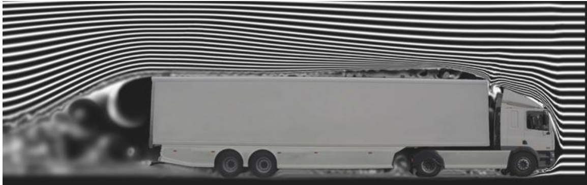
Figure 16: Example of a truck/trailer combination in a wind tunnel 37 . Specifically note the turbulent wake.
