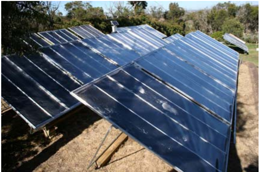
An array of Carocell solar desalination modules and a single module. (photos supplied by FCubed Ltd.)
