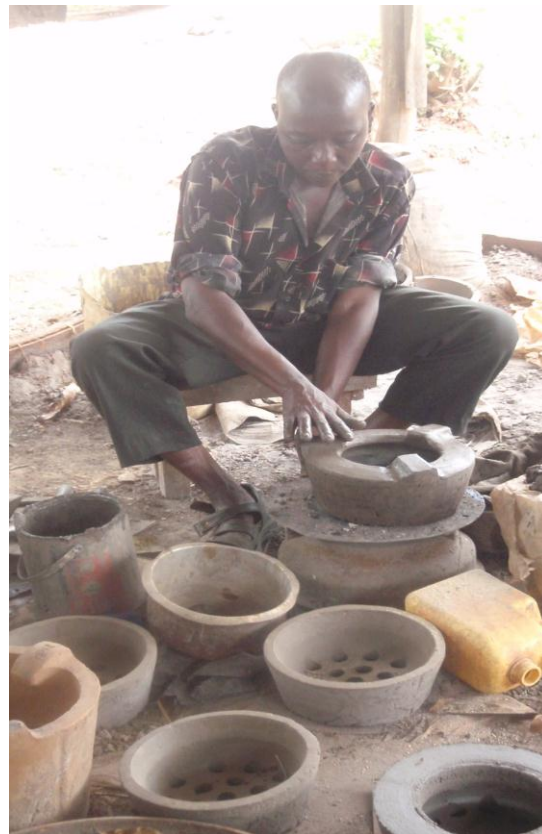
Figure 1: Joseph Muriuki fixing pot rests on an Uhai stove. Photo: Practical Action East Africa.
