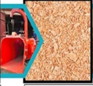
It is passed through a chipper to reduce the volume for transport o the factory
