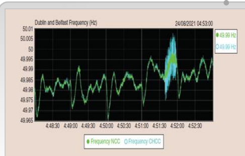
Figure 2. The oscillations transfer through a line-commutated converter HVdc line from Great Britain to Northern Ireland.
