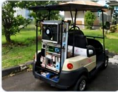
2.5 kW PEMFC Fuel Cell Vehicle + 200 WP Photovoltaic
