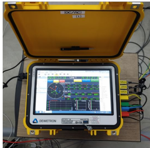
EV charging system simulator (left) / Measurement devices (Dewetron, right) Testing procedures for hybrid EV charging infrastructure
