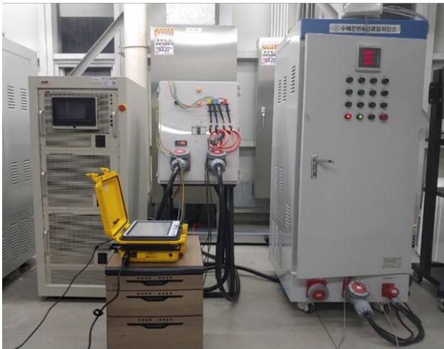
EV charging system simulator (left) / Measurement devices (Dewetron, right) Testing procedures for hybrid EV charging infrastructure
