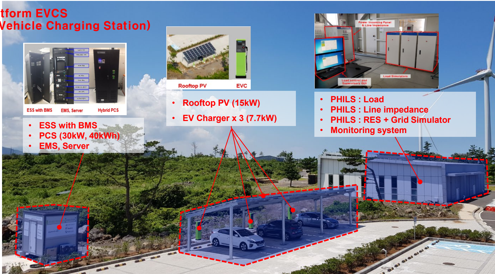
EV Charging station with RES + BESS (Jeju, Korea Institute of Energy Research)
