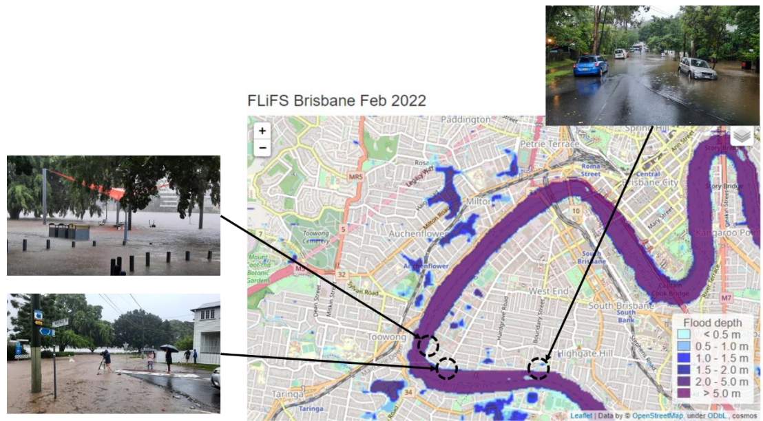
Figure 9-16. Flooding predictions by FLiFS in Australia, Brisbane during February 2022 event. Including pictures of local situation. Source: (Leijnse, et al., 2022).
