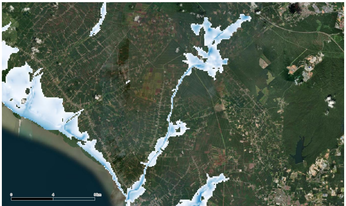
Figure 6-9 Detailed of the flood map for 2-Year Return Period for the area around Kayu Ara Pasong.
