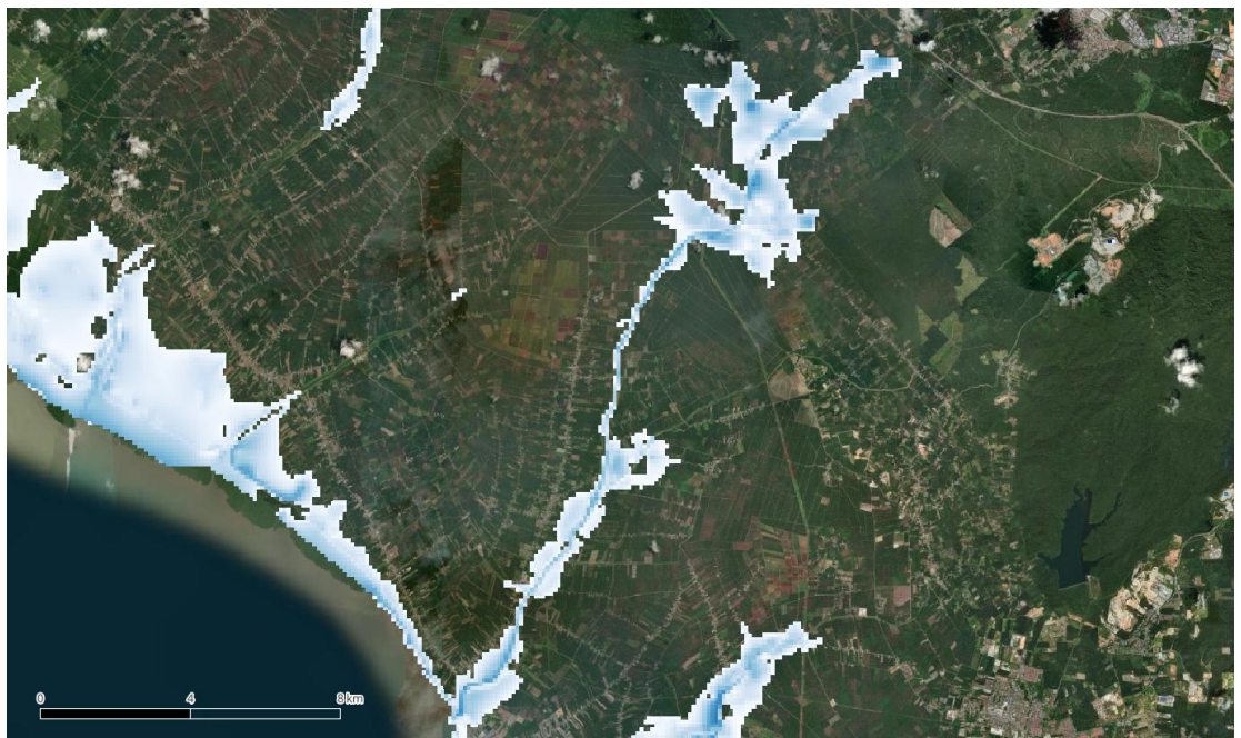
Figure 6-10 Detailed of the flood map for 2-Year Return Period for the area around Kayu Ara Pasong as an example of how the model can be used for localized hazard assessments.
