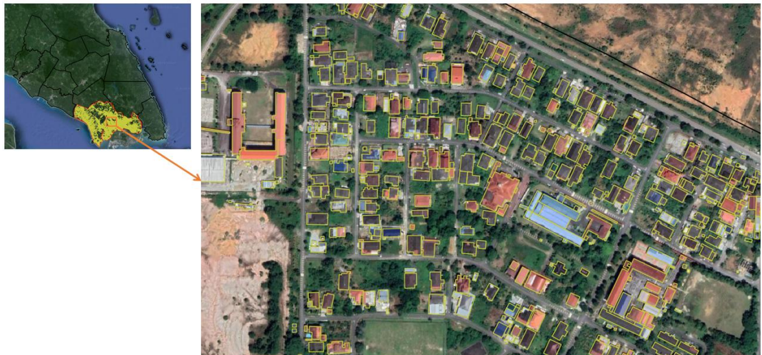
Figure 5-25 Building footprint from OpenBuilding data extent for Iskandar Malaysia.
