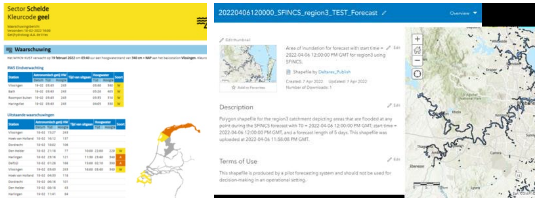
Figure 2-13 Example knowledge products for the communication of hazard information. On the left a bulletin used for communication with the public, on the right detailed forecasted flooded areas that can be used as real-time input for emergency response units.
