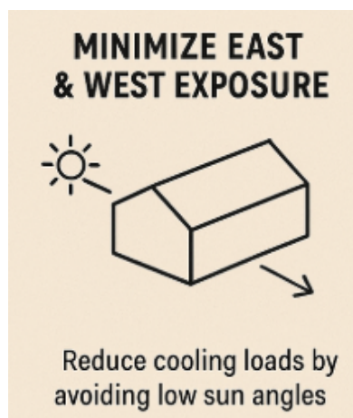
Figure 3: Minimise low sun angle exposure.
