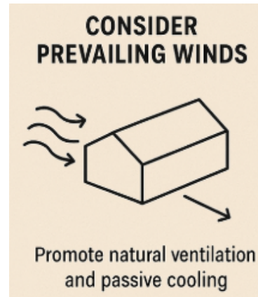
Figure 4:Using prevailing winds for natural ventilation.
