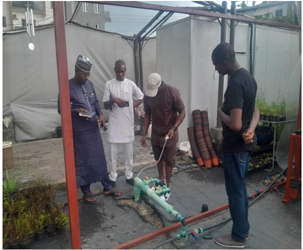
Figure 4: The Ventura pump used to optimize nutrient and water dosing
