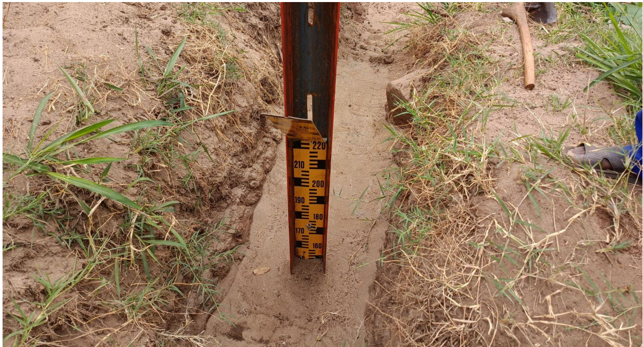
Top gauging metal plate cut and bent.
