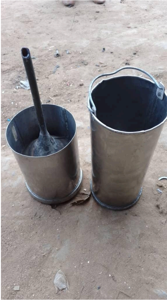
Rainfall bucket and gauge (photos pending DCCMS)
