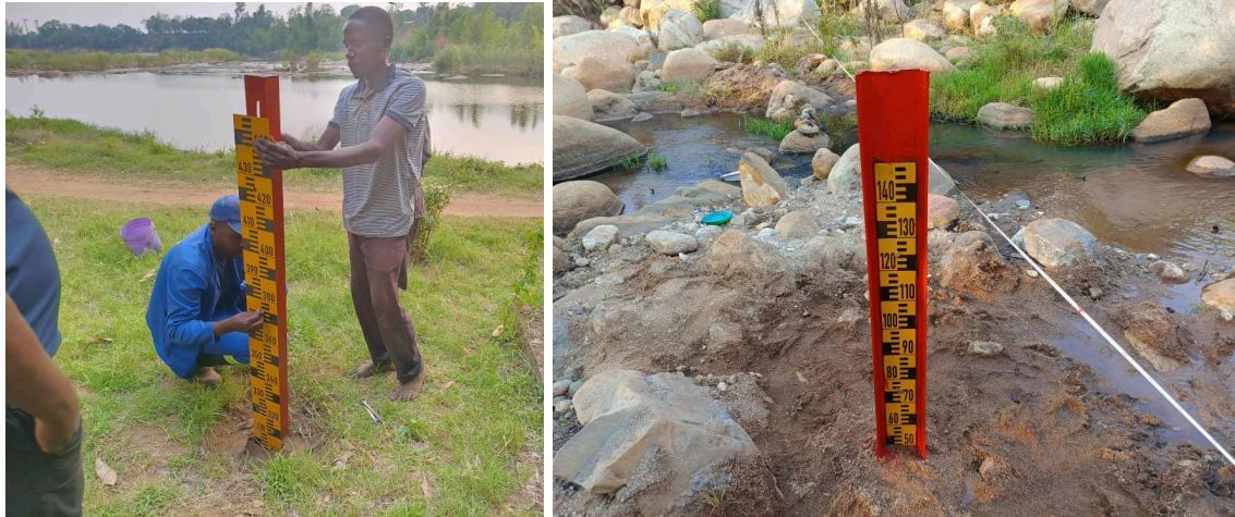
Example of river gauging plate restored at Lichenya River @ Milonde (left) and Mkwakwasi @ Mangunda (right)
