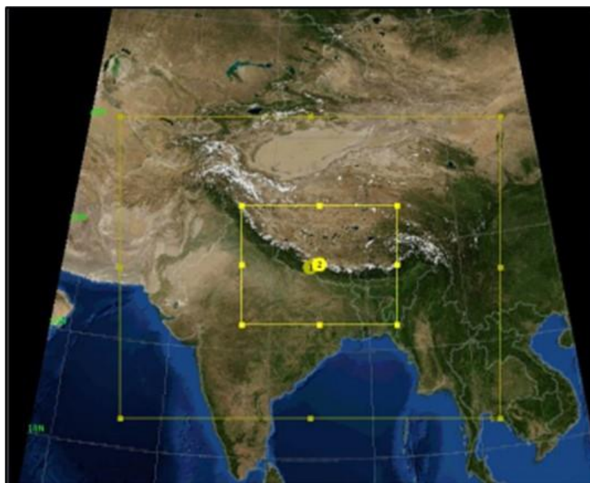
Figure 3: The WRF Model at DHM has two nested domains for the 9/3 km resolutions. The out yellow box is the 9 km domain, and inner yellow box shows the 2 ways nested high resolution 3 km domain
