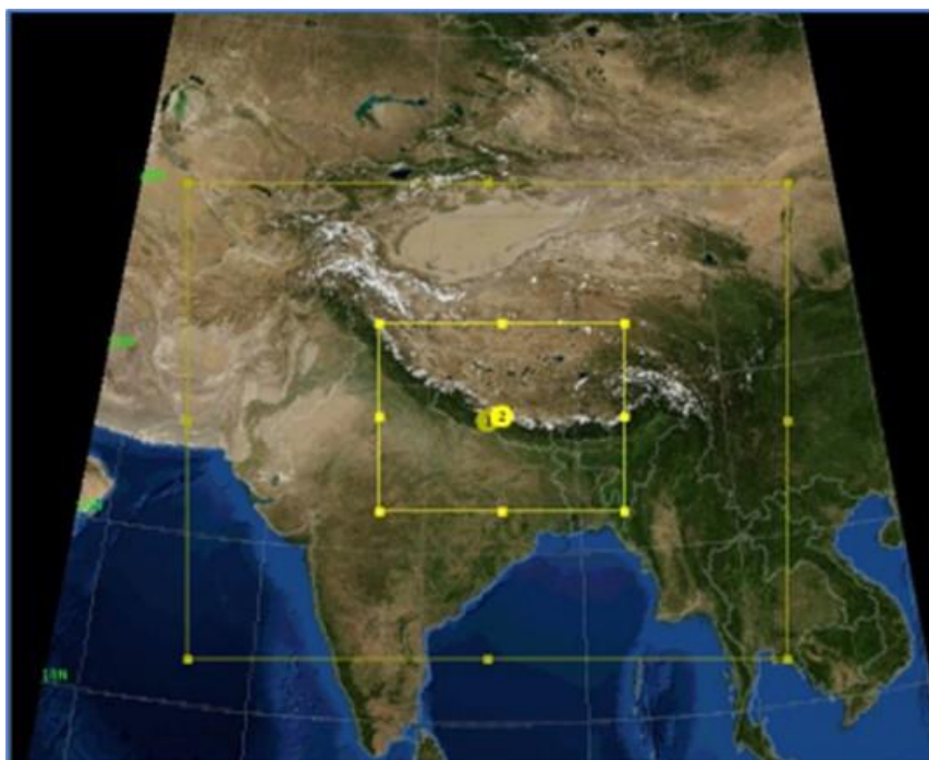
Figure 9: The WRF Model at DHM has two nested domains for the 9/3 km resolutions. The out yellow box is the 9 km domain, and the inner yellow box shows the 2 ways nested high resolution 3 km domain
