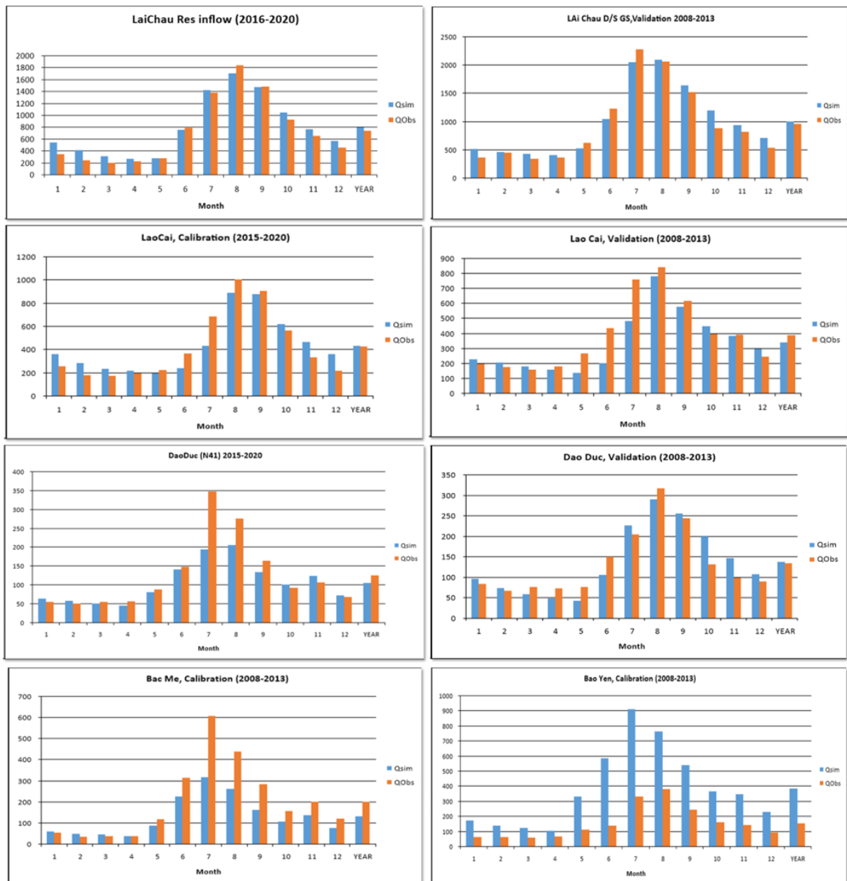
Figure 4.2 Comparison of the simulated and observed average monthly flow showing the average annual and seasonal model performance at the various gauging stations (in m 3 /s).
