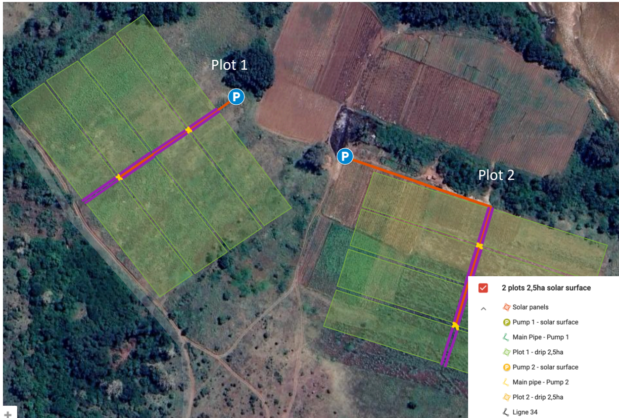
Figure 2. Geometry of the revised irrigation system in the Pangalata association.
