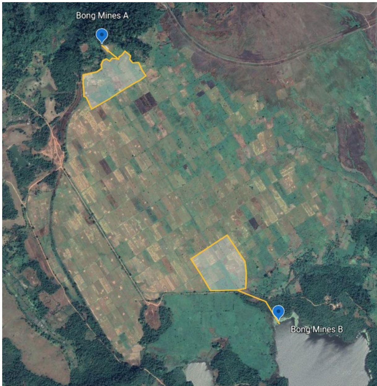
Figure 3-2 - Bong Mines Tailings Dams showing the Field Layout and two Pilot Scheme Sites
