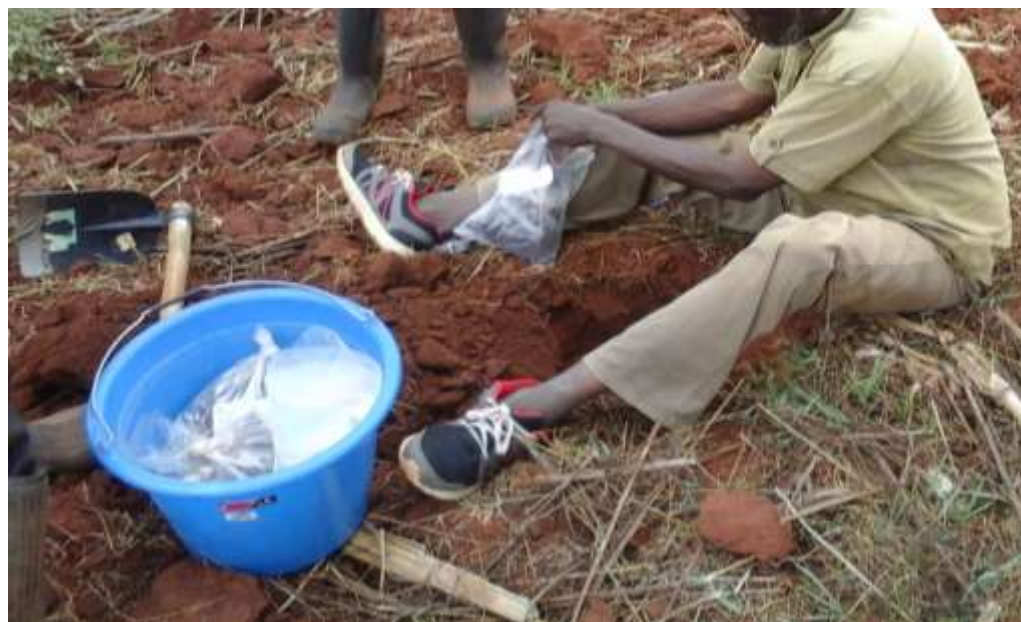
Figure 3: The soil samples should be double-bagged, labelled properly and put in the right bucket
