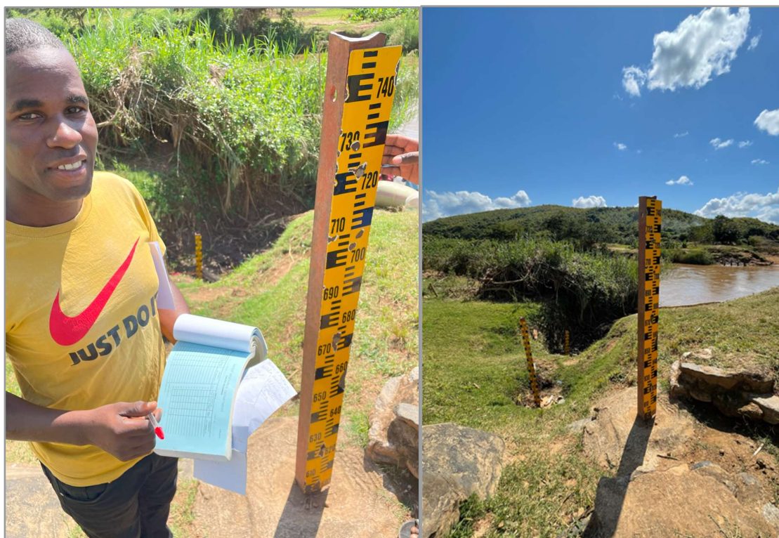
Figure 5. Manual river gauge station on the Songwe River at Mwandenga with Gauge Reader Billy Mogha showing the manual logbook for river level observations (Station ID 9B7).
