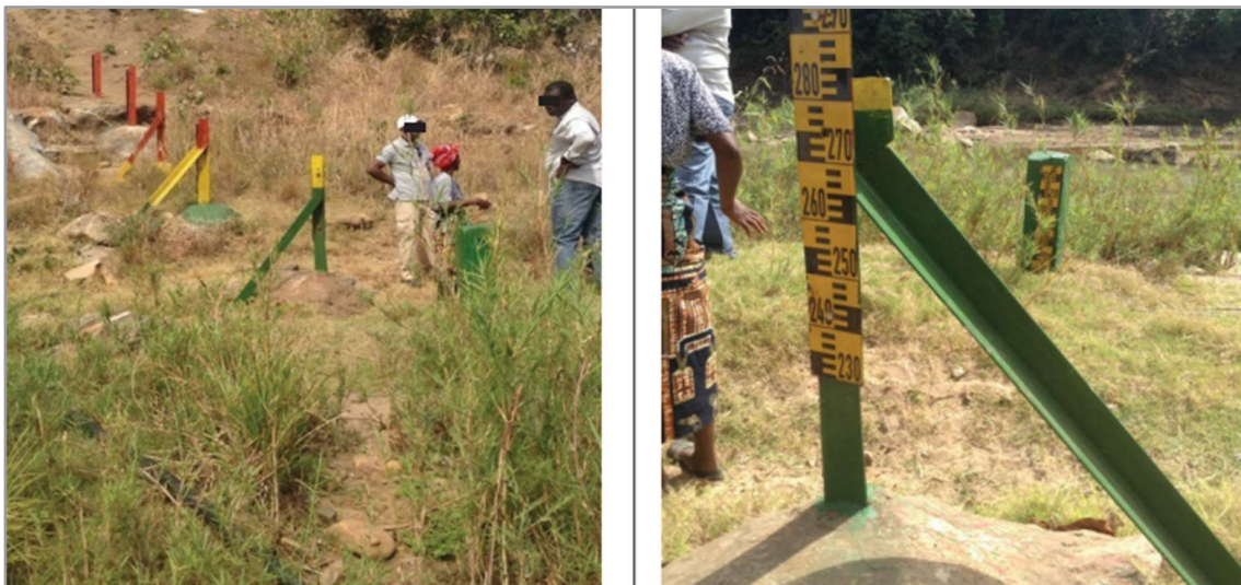
Figure 7. Example of river gauging station monitoring flood risks at threshold intervals
