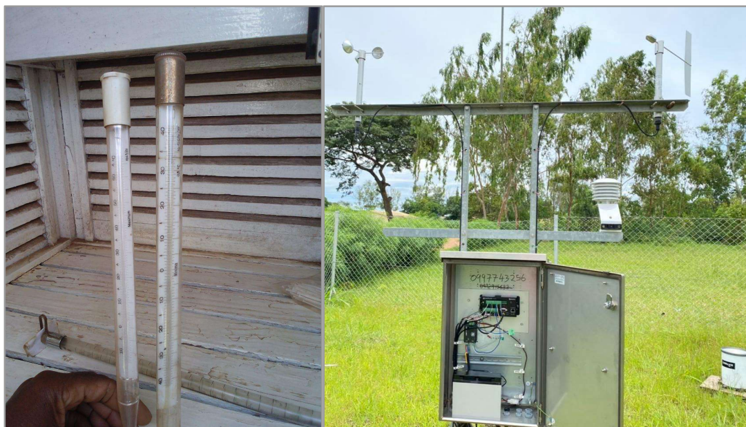
Figure 1. Monitoring equipment for collection of maximum and minimum temperature (left) and pressure, wind speed and direction (right).
