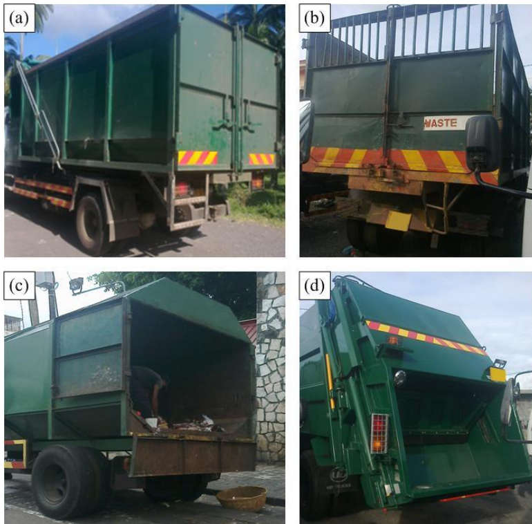
Figure 3 – Types of trucks used for waste collection in Mauritius: (a) Non-compactor truck with tarpaulin cover, (b) Non-compactor truck without tarpaulin cover, (c) Non-compactor closed truck and (d) Compactor truck
