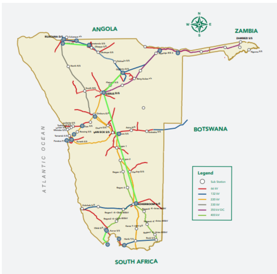
Figure 7: Generation and transmission network in Namibia. Image Source: Namibia: Geospatial Least Cost Electrification Plan, 2021
