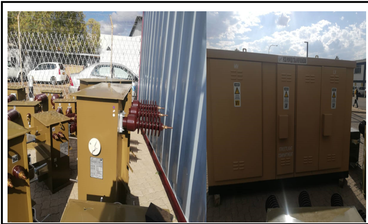
Figure 43: 10 kVA -1000 kVA single and three-phase PCB distribution transformer stock at a local supplier
