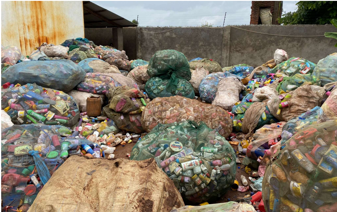
Figure 8. Rigid plastics (mainly HDPE) in 30kg bags at a local plastic manufacturer and recycler in Lilongwe (own picture)
