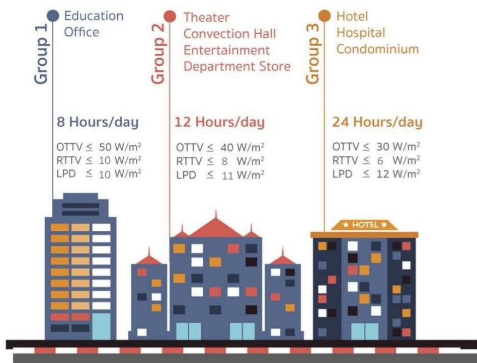
Figure 6 Basic Building Design Criteria for Different Building Types under the BEC Program
