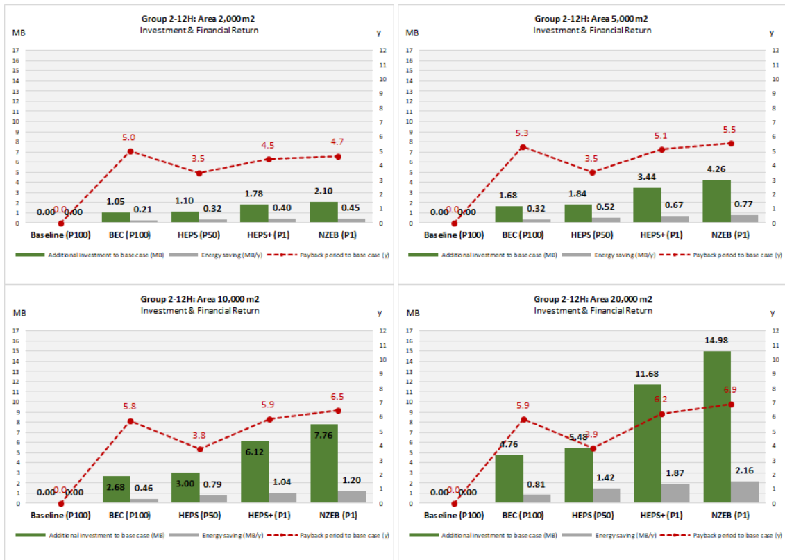
Figure 3: Investment and financial return from building envelope simulation of building Group 2-12Hr
