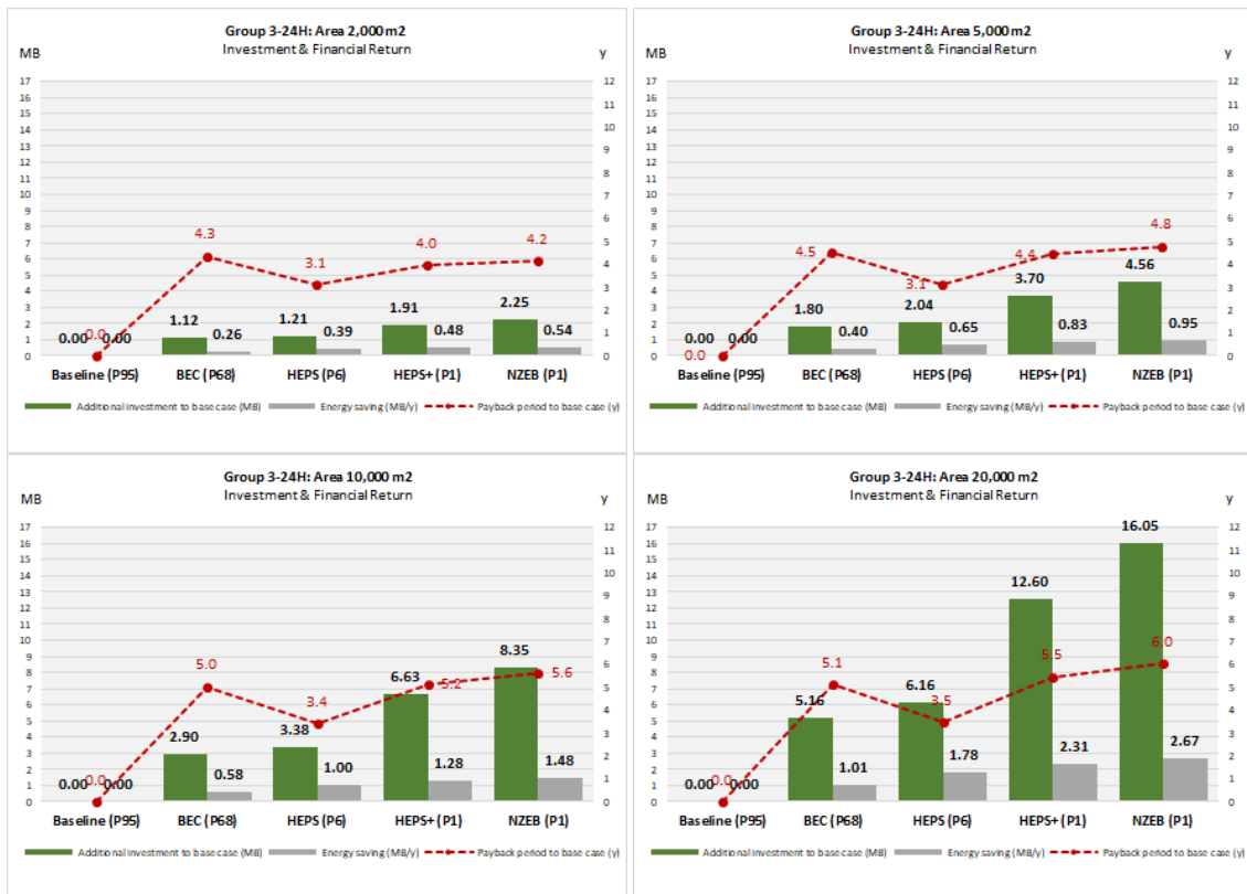
Figure 4: Investment and financial return from building envelope simulation of building Group 3-24Hr
