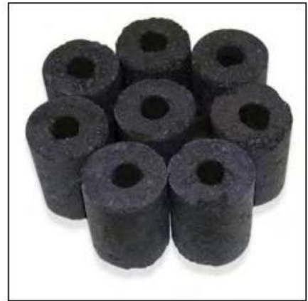
Fig. 26. (left) Screw Extruder Machine (right) Screw extruded charcoal Briquettes (Singh, 2010)
