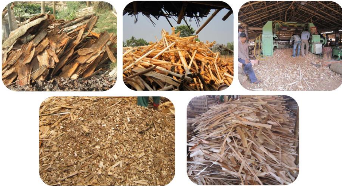
Fig. 47. The various waste obtained from the Shree Hari Om Veneer Udyog factory (clockwise from top left): Bark; Remaining Central Part ( golla/gollia ); Sawdust; Small Pieces of Wood; and Unusable Veneer (CEEN, 2014)
