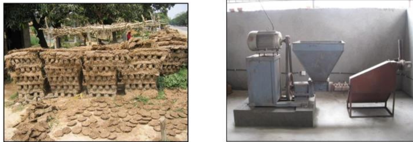
Fig. 38. (left) Guitha - Traditional Animal Dung Briquettes used in Nepal and (right) Rice Husk Briquetting Machine in Nepal
