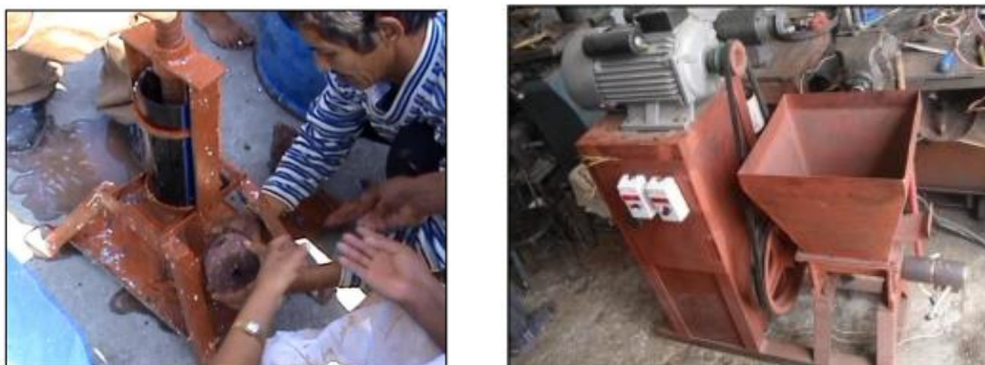
Fig. 41. (left) Compression Briquetting of Waste Materials by FoST and (right) Portable Screw Extruder Briquetting Machine
