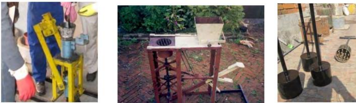
Fig. 30. (left) Improved hand mould (centre) Foot peddle press mould (right) Chinese manual mould
