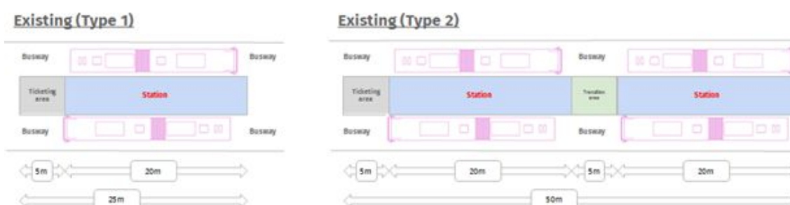
Figure 32 Existing Transjakarta Station Design
