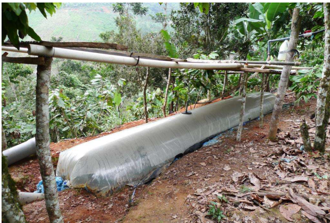
Figure 1: Botero & Preston biodigester operating for 3 years in Las Lajas in 2013 (El Oro).
