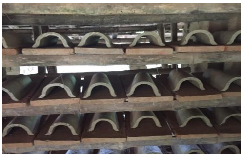
FIGURE 60 CURING AFTER MOLDING (LEFT AT ROOM TEMPERATURE FOR TWO DAYS)
