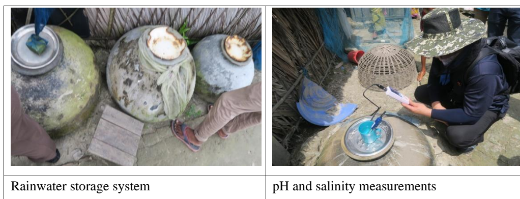
FIGURE 16 DRINKING WATER STORAGE SYSTEM AND SALINITY MEASUREMENTS
