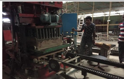
FIGURE 52 BRICK MANUFACTURING PROCESS BY VIBRATIONAL MOLDING
