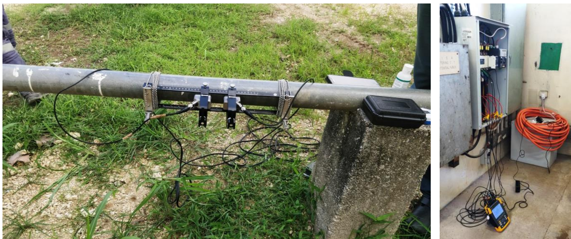
Figure 12 Water flow and power measurement photograph
