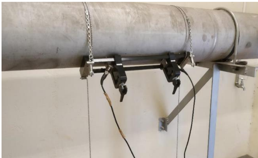
Figure 12 Water flow measurement photograph
