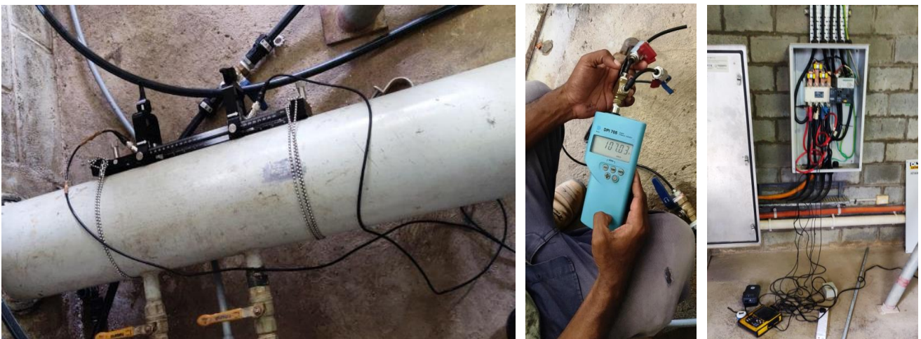
Figure 12 Water flow, head and power measurement photograph
