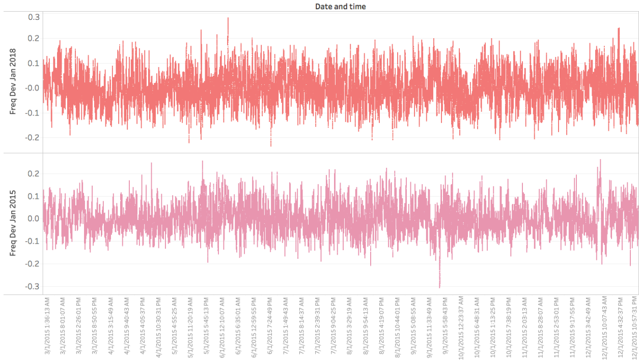
Figure 3. Frequency deviations for the first two weeks in the month of January in the years 2015 (bottom) and 2018 (top), in the National Grid system (Data source: National Grid)
