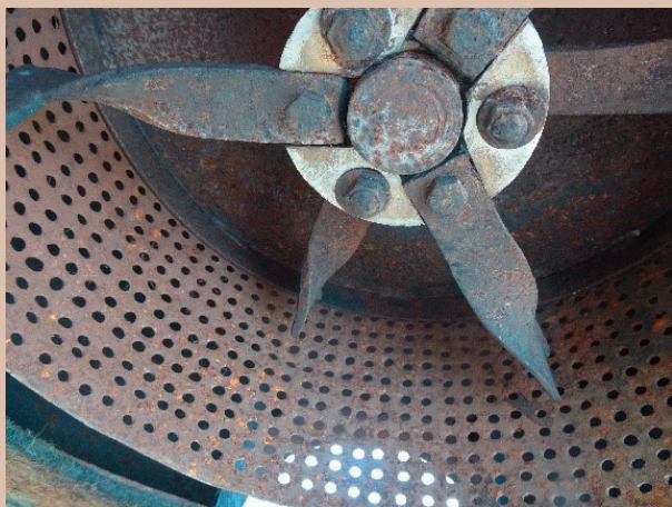
Picture 5: Hammermill, milling chamber
