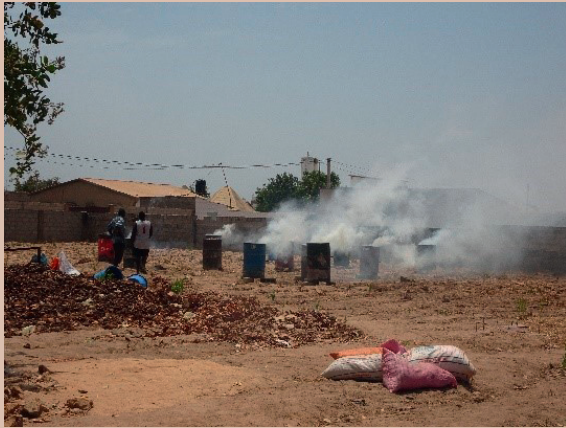
Picture 6: Carbonization process, drying phase
