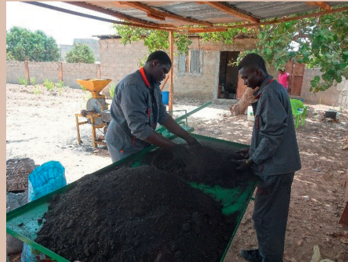
Picture 15: Pyrolyzed powder and binder mixing
