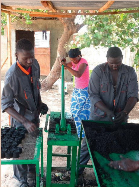
Picture 19: While one cup is pressed, another one is filled and the third one is emptied:
