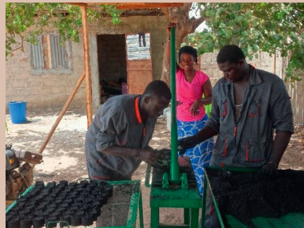
Picture 18: One cup is taken out the press, while another one is placed.
