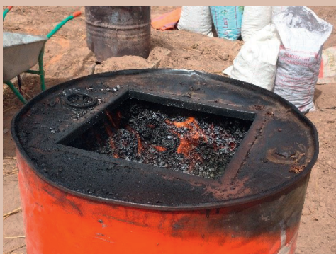
Picture 7: Groundnuts carbonization, methane burning
