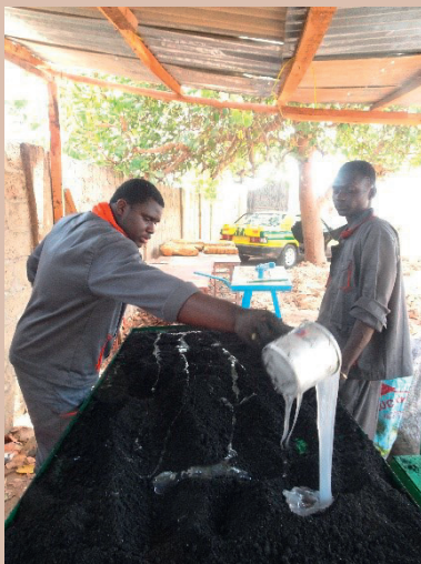
Picture 16: Binder mixing with milled groundnut shells (2)
