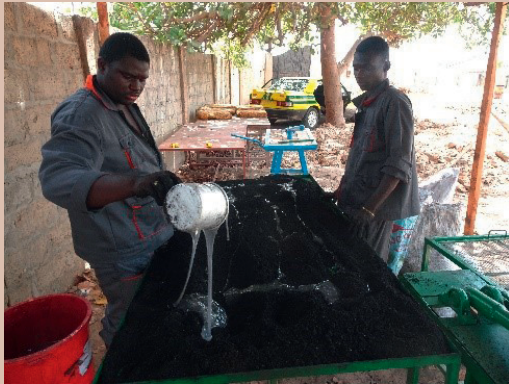
Picture 14: Binder mixing with milled groundnut shells (1)
