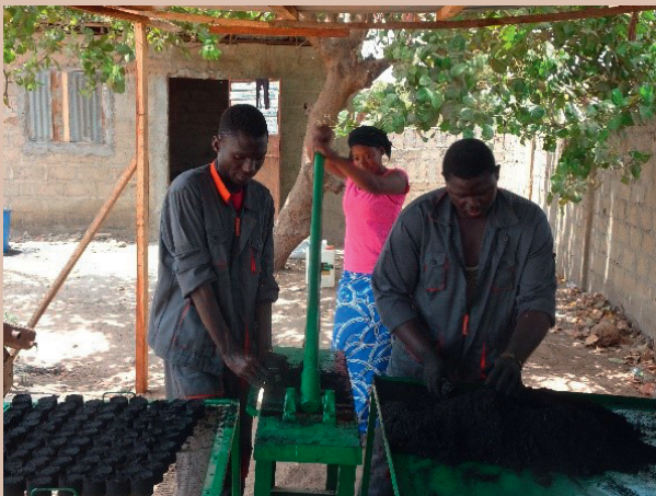
Picture 17: One cup is filled with the Mix, while one briquette is pulled out another cup and arranged on the drying tray.
