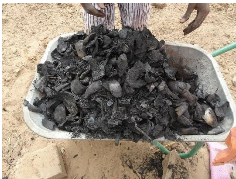
Picture 24: Pyrolyzed coconut shells
