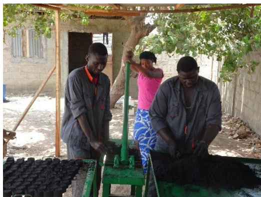
Picture 33: One cup is filled with the mix, while one briquette is pulled out another cup and arranged on the drying tray
