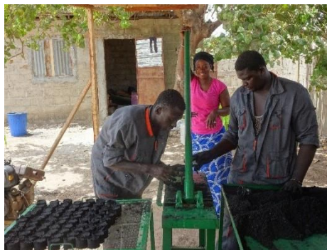
Picture 34: One cup is taken out the press, while another one is placed
