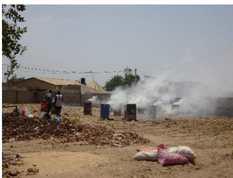
Picture 20: Carbonization process, drying phase
