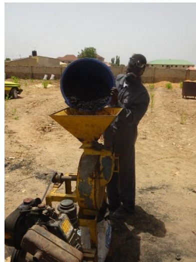
Picture 28: Hammermill, productivity test
