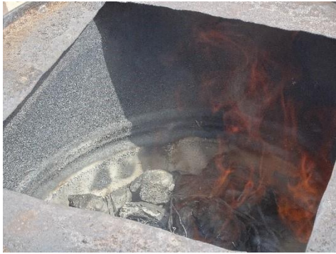
Picture 22: Coconut shells carbonization, methane burning
