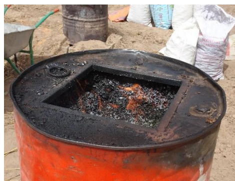
Picture 21: Groundnuts carbonization, methane burning
