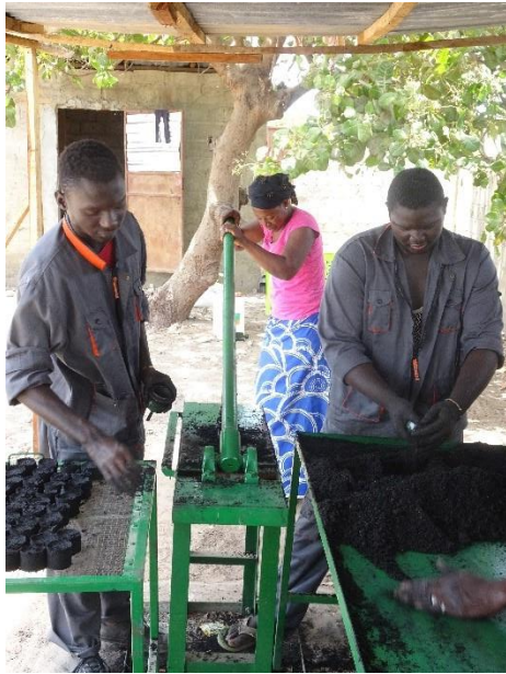
Picture 35: While one cup is pressed, another one is filled and the third one is emptied
