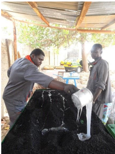
Picture 31: Binder mixing with milled groundnut shells (2)
