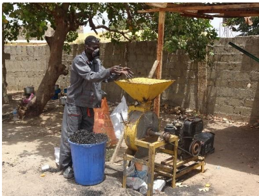
Picture 27: Hammermill, productivity test
