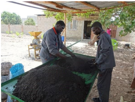
Picture 32: Pyrolyzed powder and binder mixing
