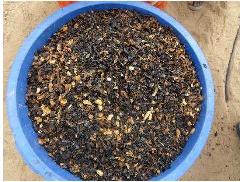
Picture 23: Partly pyrolyzed groundnut shells
