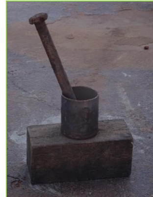
Picture 8: Hammer & piston briquette production technique - 2
