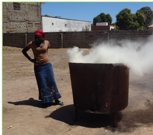
Picture 9: Open barrel pyrolysis (burning) technique
