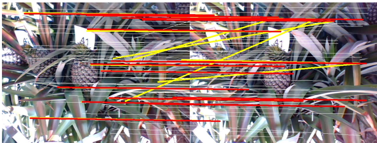
Matching of SIFT interest points for two frames of a field video.
