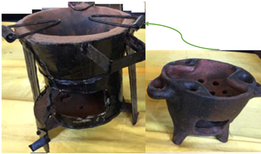
Figure 2. Metal stove with a clay liner produced during the project by a female clay stove producer (Wasiya Abdallah) and male metal stove producer (Baldwin F. Mpunga).
