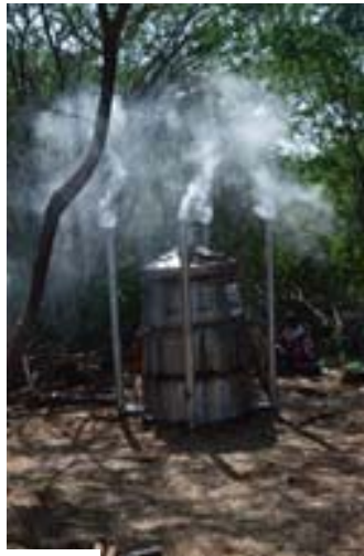
11. Steel ring kiln, Turkana Photo by J. Owino
