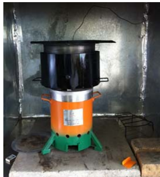
Figure 19 Ceramic lined gasifier by KIRDI. Technical drawing by Barbara Njeri
