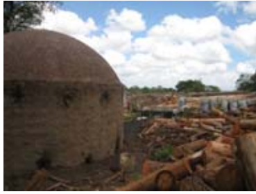
Figure 10. Masonry high efficiency improved mound kiln used at Kakuzi Ltd, Thika, Kenya.
