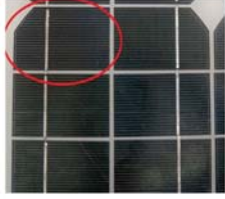
The circled cell is a different shape and size than the other cells having full corners.
