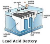
Lead Acid Battery Source: Gravita Technomech
