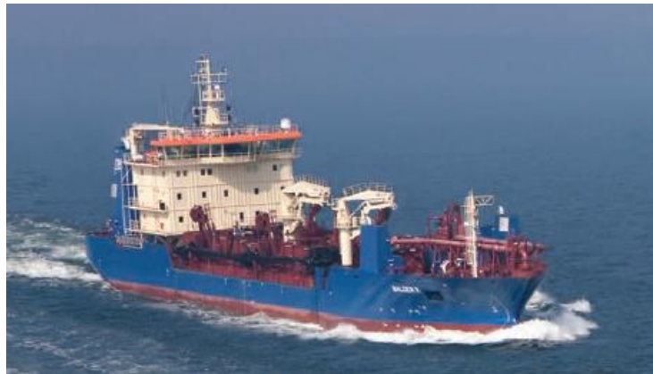
Figure 3.1 Modern hopper suction dredger with a capacity of 5000 m 3
