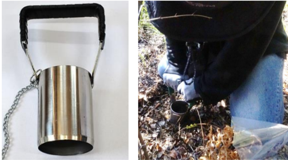
Fig. 2. Collecting soil samples using soil core sampler
