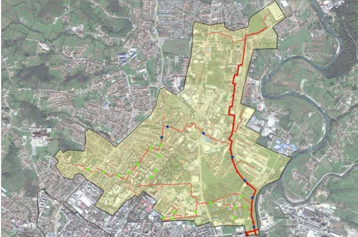
Figure 40: Reconstructed Part of “Industrija” Pipeline
