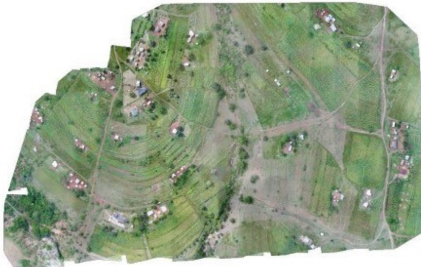
Figure 9: A sample RGB orthomosaic image after processing UAV images from multiple flight missions.
