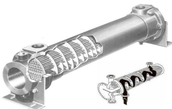
Figure 8.10: Shell-tube heat exchanger with one pass
