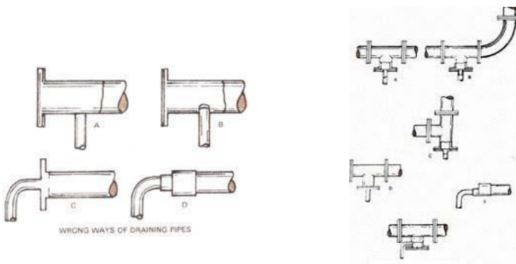
Figure 3.10A: Wrong ways of draining pipe Figure 3.10B: Right ways of raining pipe
