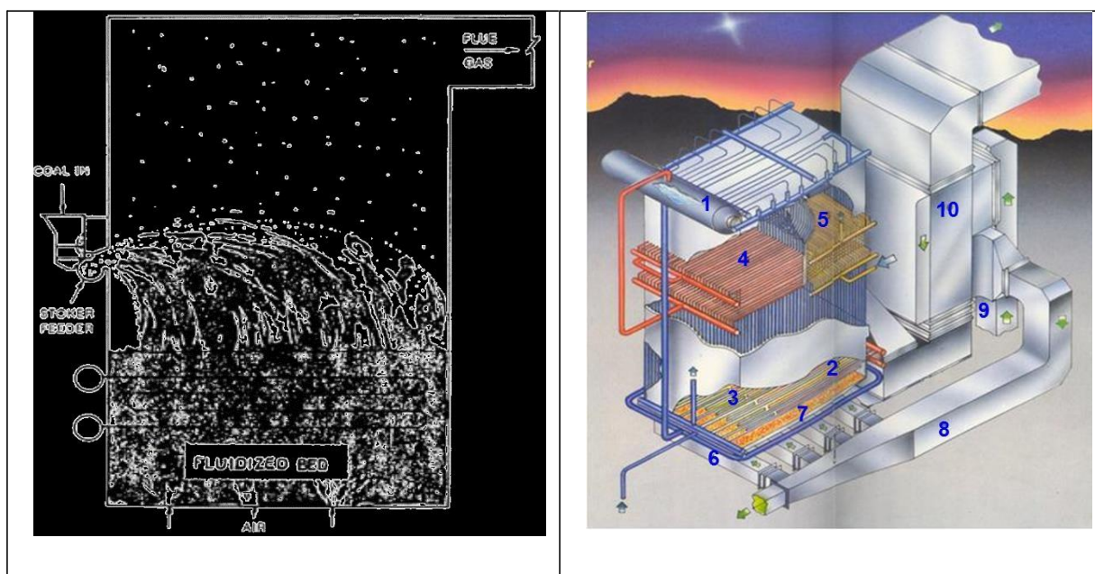
1 Steam Drum, 2 Bed Super-heater, 3 Bed Evaporator, 4 Convection Super heater, 5 Economizer, 6 Wind box, 7 Air Distributor Plate, 8 Hot Air Duct, 9 Cold Air Duct, 10 Air Preheater
